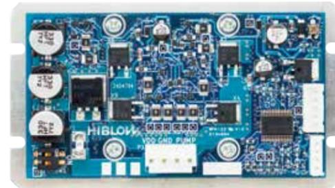
The HIBLOW Driver System consists of an inverter (PCB) board and a heat dissipation frame.
